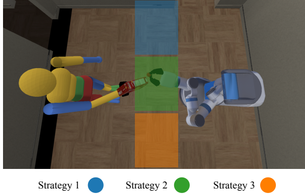
Figure 6: HR-Handover. We classified handover regions into three categories for post-hoc analysis. The classification is based on the relative location of where the handover happens in front of human. From left to the right, they are strategy 1, 2 and 3.
